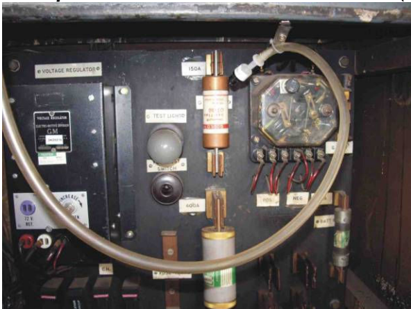
Cabin fuse & battery knife switch backing board in a Y class locomotive
